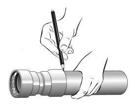
A permanent marking on the PCC system pipe (or insert adapters, street bends f/m or male and crossover bends) is required to make a solid press connection. This marking is to be applied before attaching to the end of the pipe.
